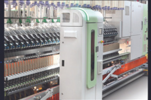
Ring Frame Auto Piecing Automatic piecing for higher productivity and superior quality
