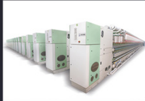
LRJ9/SX Smart Ring Frame with integrated suction compact system for superior quality
